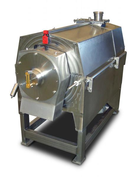
High quality and performance solid - liquid separation system by perforated mesh and helical paddles rotating at high speed, driving the product for sieving.
