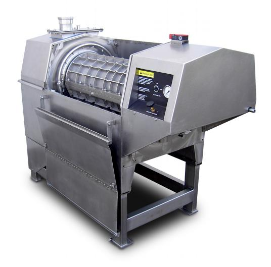
High quality and performance solid - liquid separation system by rotating auger and perforated mesh, dragging and pressing the product throughout its length.
