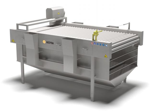
Allows manual selection and elimination of poor quality fruit for processing.
