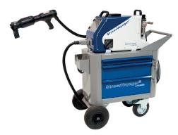
Portable and compact shot peening system - STRESSONIC® technology
