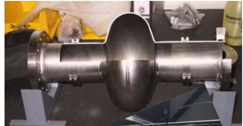
CAVITIES (for accelerators) made from Nb = Niobium
