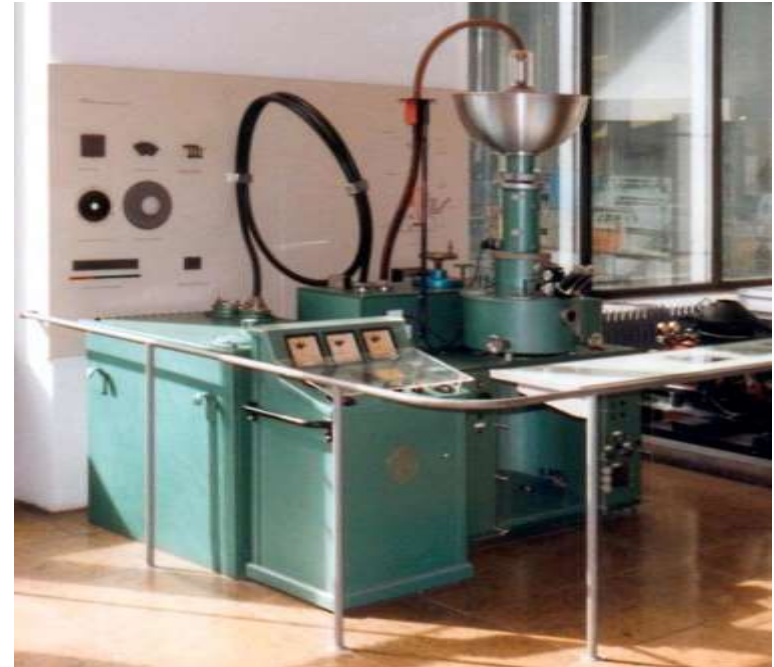
1958: The first electron beam welding machine (55kV) manufactured by Karl-Heinz Steigerwald.
