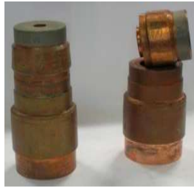
Electrical contacts Made from Tungsten and Copper
