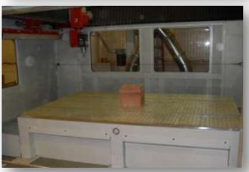
Conventional steel frame table, aluminum vacuum table or T-slot. Clamping systems suitable for any part fixturing need
