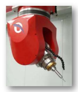
**Belotti FORK head** is designed and patented by Belotti. The cast iron yoke type head is equipped with torque motors, one for the fourth axis and two for the tilting axis, independently cooled. It can fit either a 20kW Fischer electrospindle at 30.000rpm or a 40kW electrospindle from IBAG at20.000rpm and 50Nm (S1) torque
