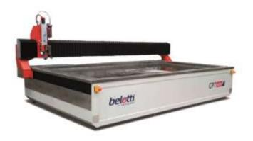
The cutting can be performed either with pure water or with abrasive to increase the erosion power of the water on large thickness as well as metals, potteries, rock and bullet-proof glass
