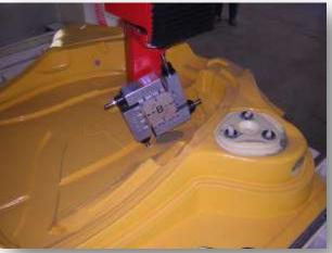
Trimming of large-sized thermoformed materials
