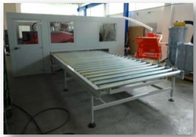
Belotti automatic loading & unloading conveyors allows a faster piece positioning in order to reduce cycle times
