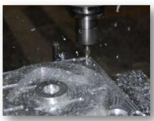
Milling test on 5 axis NAS
