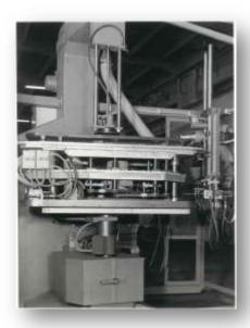
1982: First CNC machine with 2 axis (X-Y) for panel milling. It is equipped with a CNC BOSCH
