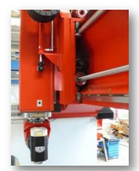
Motion driven by recirculating ball screws diam. 50mm pitch 40mm on the 3 linear axes, closed loop feedback with 5 micron accuracy **Heidenhain linear scale**
