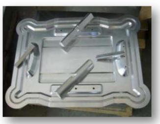
Aluminium mould milling
