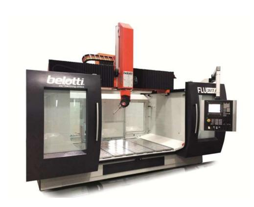
The new machining center Series **FLU** built with monolithic structure to dampen vibration, is intended for high-speed milling of resin models and aluminum moulds. The special architecture of the machine allows a total accessibility to the working area, with the possibility to load jigs and pieces using a crane.
