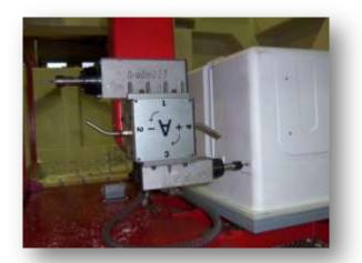
Revolver type: from 2 up to 4 electro spindles from 1 to 4 kW. It allows a very quick tool change, less that two seconds.
