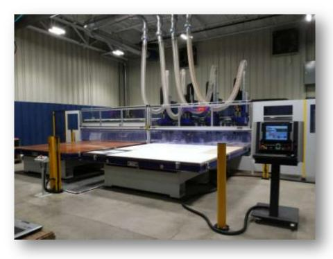
**Gemini** series CNC machining centres are the result of Belotti S.p.a. long experience achieved in more than 30 years of activity in the production of machines for aluminum, composites materials and resins milling applications. Machine construction shall consist of an heavy-duty, reinforced cast iron and stress relieved steel weldment, together for machine stability.
