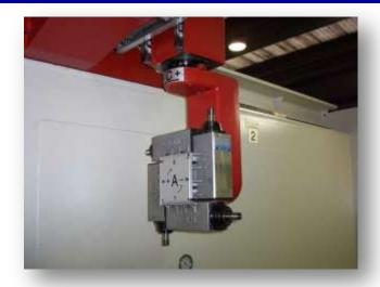
Machining unit with 4 independent electrospindles
