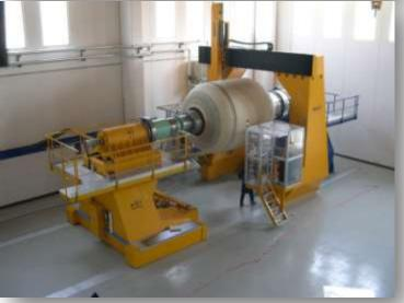
**VEGA Series** machines are 5-axis simultaneous CNC low driven portal Gantry machining centres combined with a lathe system made of headstock/tailstock.
