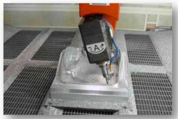
Aluminium mould machining
