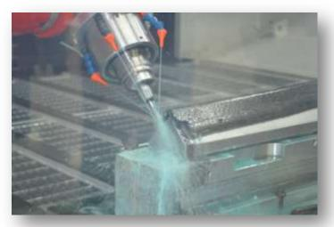
Carbon fiber machining with coolant
