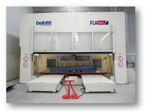
In addition to standard fixed table, special loading/unloading systems may be provided as carousel rotary table and single or twin shuttle systems
