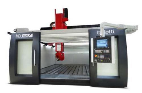
The MDL series ensures maximum productivity when milling models and prototypes as well as finishing of large-sized moulds and aluminum/composite aerospace parts. 5-axis heads equipped with torque motors, linear scales on the linear axes and high rigidity frames enhance the machining accuracy and finishing quality.
