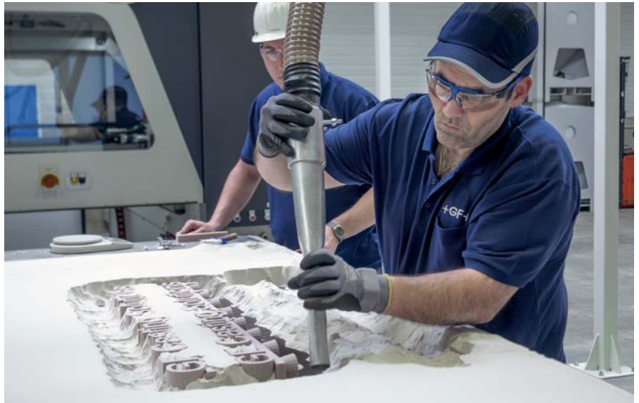
Figure 9 Post-printing: Vacuuming non-bonded sand
