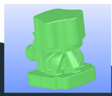
A complex dirt bike cylinder that ties together the water jacket, intake, and exhaust has been cast with 3D printed cores in production since 2015. Annual design changes are incorporated without hard tooling investments.
