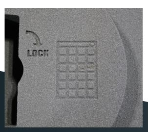
With the flexibility of additive manufacturing design, Hoosier Pattern can print lift holes for part handling (left) or their quality audit grid and, when needed, assembly instructions, onto each part to help ensure all process steps have been completed before shipping a core to a customer (right).
