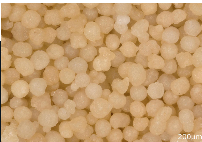
Kimura developed a patented artificial ceramic sand for increased casting quality. The samples to the right show a silica sandcasting with veining defects (left) and a defect-free casting (right) using Kimura’s ceramic sand.
