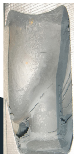
Kimura developed a patented artificial ceramic sand for increased casting quality. The samples to the right show a silica sandcasting with veining defects (left) and a defect-free casting (right) using Kimura’s ceramic sand.
