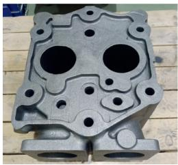
A traditional replacement casting carried a 10 month lead time for tooling — this replacement was produced with sand 3D printing and delivered in weeks
