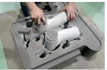
Speed 3D Mold used it's S-Max® sand 3D printer to create a pattern and core box set from a CAD file without tooling
