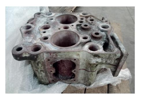
A replacement for this cracked cylinder head was needed to return a cargo boat to service, but no casting pattern existed
