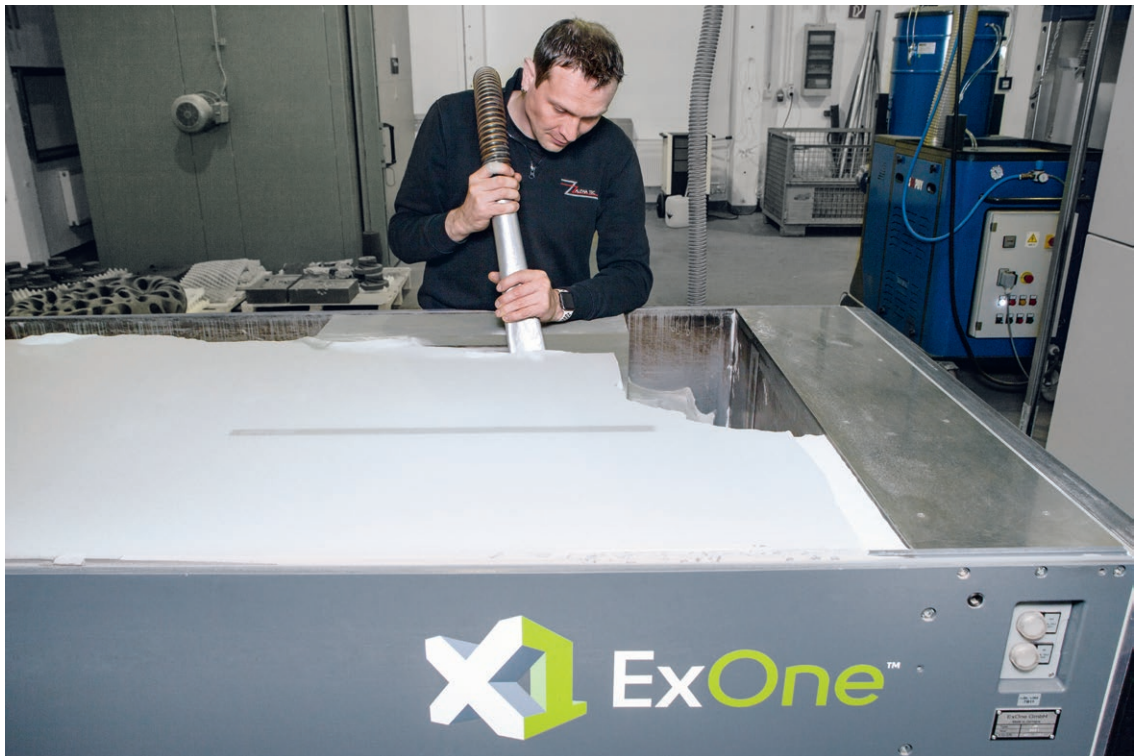
Post-printing; vacuuming non-bound sand
