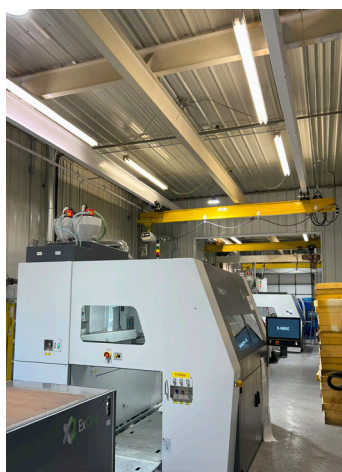
Austin T. Crawley walks through the Dundee Castings sand 3D printing building where two S-Max Pro binder jetting systems produce seat foam molds and other complex geometries.
