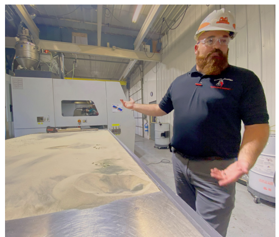
Austin T. Crawley walks through the Dundee Castings sand 3D printing building where two S-Max Pro binder jetting systems produce seat foam molds and other complex geometries.
