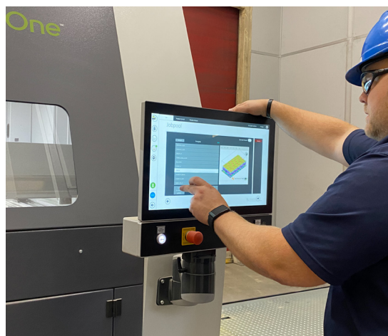
Engineer Kyle Peterson operates the ExOne S-Max Pro at Grede. Job box allocations are optimized to fit several hundred cores into one build
