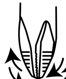
**ACR** stands for the "anti-camout ribs" that are formed on screw driver tips and may also occur in screw sockets. The ribs adhere securely to screws to minimize camout while reducing worker fatigue. ACR drivers can reduce camout by 30% to 40%.
