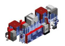
Presentation: automatized cell with EDM and milling machine, 2 *Chameleon* Quad – conntected with a *Chameleon* linear version
